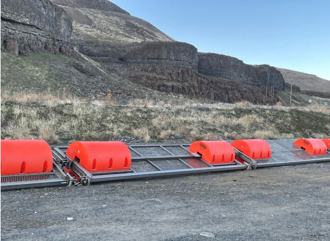
Image 2. Multiple sections of the fish ladder exit debris barriers assembled on shore.
